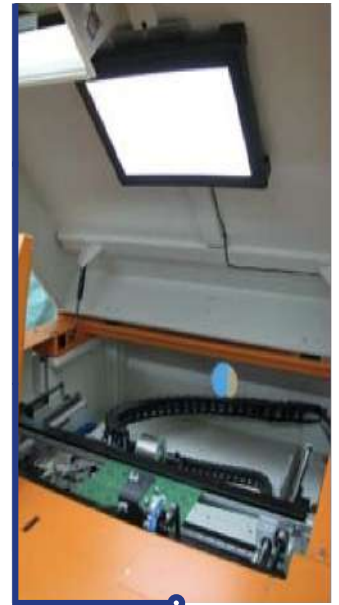
Pre-heaters for high thermal mass boards
